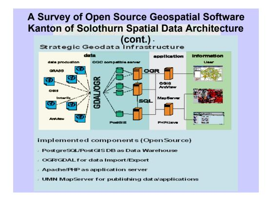
Here we see an architectural diagram showing the data residing in PostgreSQL/PostGIS databases being served by Apache and PHP and being transformed using GDAL/OGR
