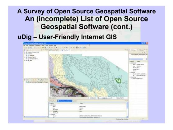
This shows uDig with the Duck Mountains East contour SHAPE file (from Manitoba) opened with one contour polygon selected for editing. The polygon attributes are shown on the right side of the window and the bottom of the window shows the attributes and the coordinates.
