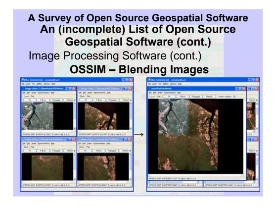
OSSIM provides three ways of combining images, mosaicing, blending and feathering which allows for a variety of effects when combining images. The image on the right has been feathered.
