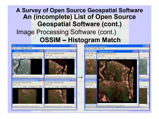
Here OSSIM is matching the image colours of four images together. The first image opened is the one that others are matched to. There should be some overlap between the images in order for this matching to be performed well.
