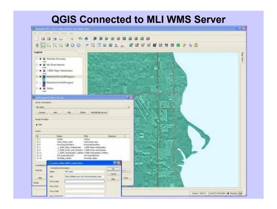
The MLI WMS connection and layers are shown here. There are several MLI WMS layers displayed with the Orthophotography layer at the bottom and a 10Km grid with transparency set shown above it and the 1:500K water layer from the WMS server and the MLI road network shown above that. This is the same MLI WMS data that was shown earlier in the browser capture.
