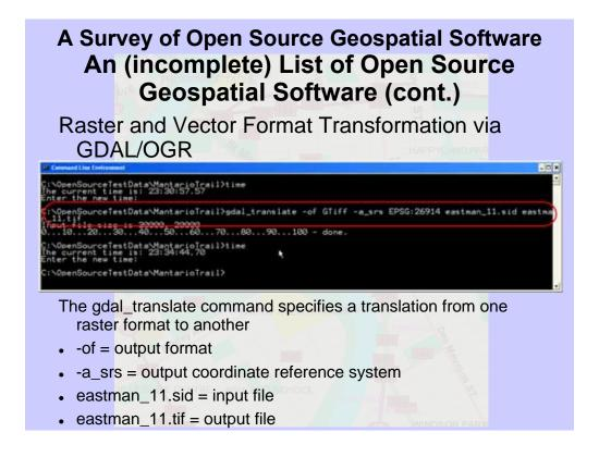
This instance of the gdal\_translate command translates from MrSID format to GeoTIFF format specifying that the output image is in the EPSG 26914 coordinate reference system (NAD83 UTM Zone 14)
