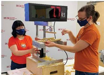
Nhi Le, P.Eng., and Ronnie Sugden, P.Eng., testing the load of trusses made of spaghetti and white glue.
